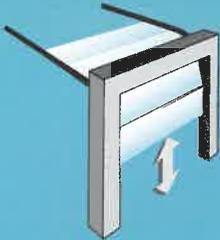
A 3D diagram of a sectional garage door mechanism, showing the door panels and the internal structure. The diagram is set against a blue background.
